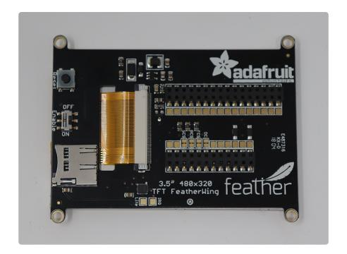
After that, it's just a matter of inserting the Feather M4 Express into the back of the TFT FeatherWing.
