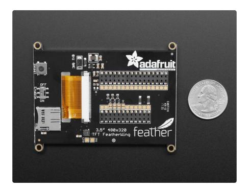
This Wing comes fully assembled with dual sockets for your Feather to plug into. You get two sockets per pin so you can plug in wires if you want to connect to Feather pins. Alternatively, each pin has a large square pad on the PCB for direct soldering.
