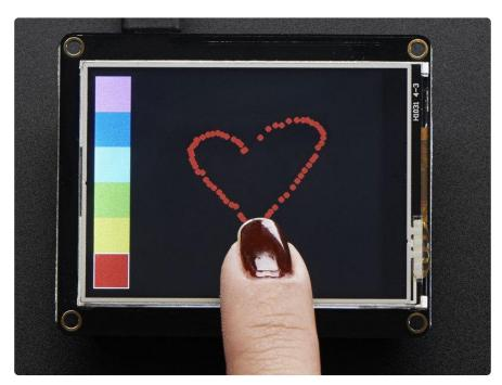
The touch screen is made of a thin glass sheet, and its very fragile - a small crack or break will make the entire touch screen unusable. Don't drop or roughly
