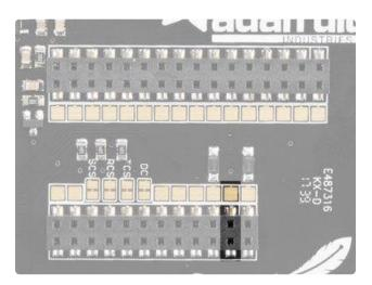
You can turn off the 3.3V power supply with the EN pin or the switch attached to that pin. The enable/disable switch on the bottom of the Wing will also deactivate the backlight
